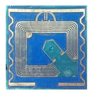
ALL-TAG's 2in1 Label combines RFID and Electronic Article Surveillance (EAS) technologies in a single label. The labels are compatible with UHF RFID readers, and 8.2 MHz EAS systems and deactivators. The 2in1 Label provides retailers with a simple and cost-effective solution for tracking merchandise, improving inventory management, and decreasing shrink.
